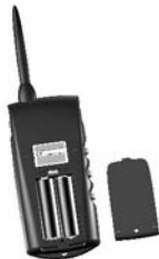
Replacing batteries of CANICOM 1500 remote control Diagram 10
